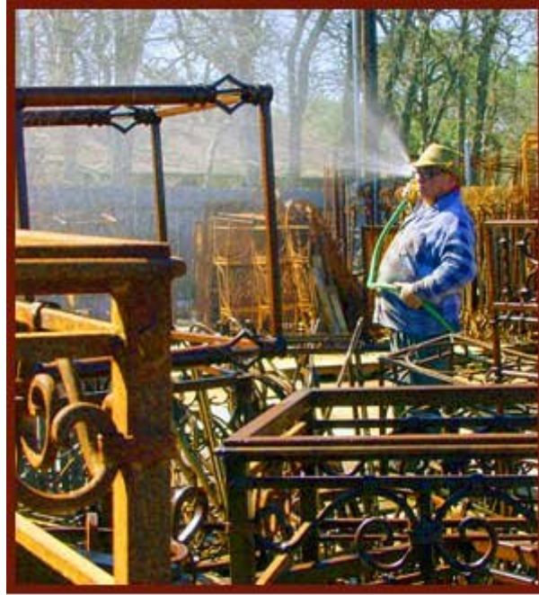
Jose tends to the "rust garden" in Boerne, Texas. This is where iron product is oxidized before being treated to an industrial sealer to create the Natural Rust Finish.
